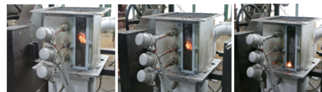
Fig. 140 Visualization of the sintering zone through the heat resistant transparent wall (Slovakia)
