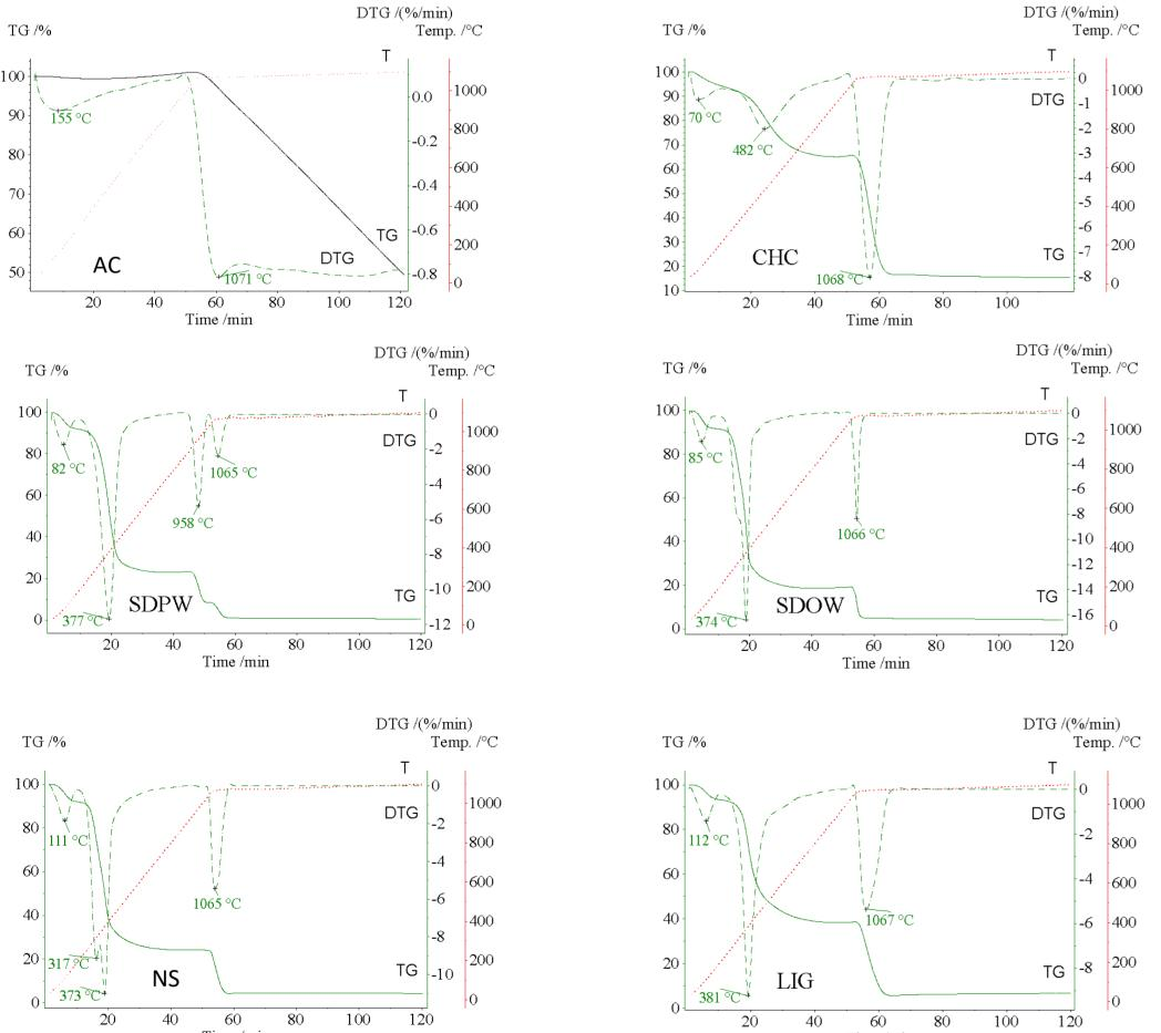
Fig.3 TGA plots of biomass samples and BF.coke
