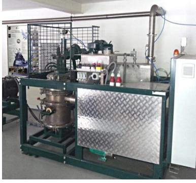
Test the influence of the quantity and flow of hydrogen on the reaction mechanism of Mn ore, test the impact of hydrogen on the quantity and chemical composition of Mn alloys, examine the effect of hydrogen on the quantity and composition of process gases.
