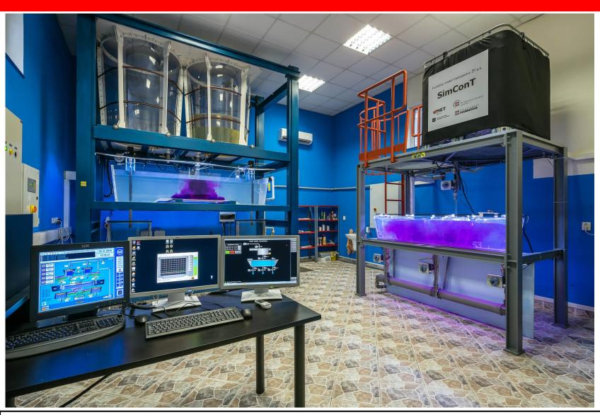
modelling of liquid steel flow processes in continuous casting
