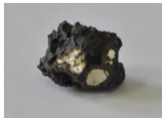
Figure 2 Free lime in the slag at the end of oxygen blowing. Melting process S2.
