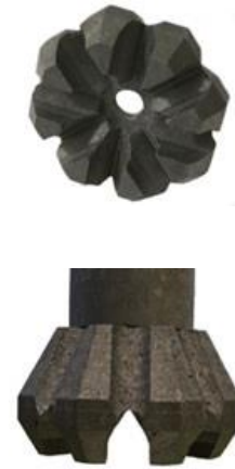
Figure 2 Detail of the impeller head used for physical modelling, variant J8.
