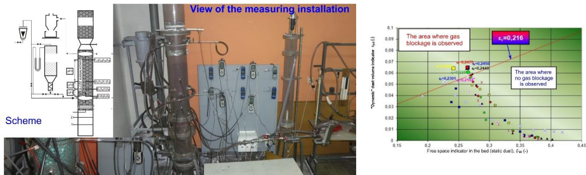
Figure 3 View of the third generation installation and the criterion determining the moment of blockage of two-phase flow (gas + dust) through the packed bed.
