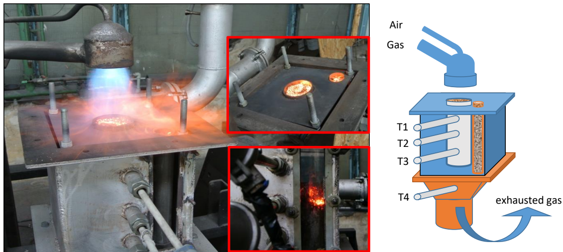
Figure 1 Laboratory sintering pan modification for experimental works.
