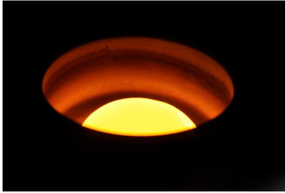
Figure 3 Picture of aluminium surface melted with 15kW of power emitted in the deposit.
