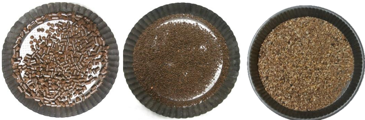
Figure 2 Black pellets (left - as received, middle-fraction after disintegration) and final MgO inert material (right).
