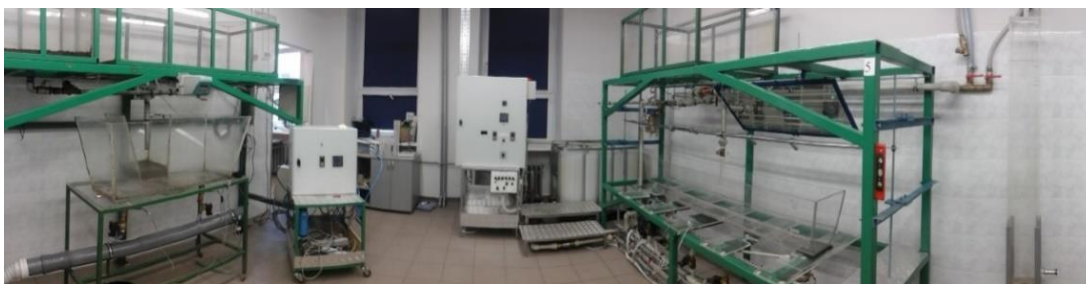
Figure 2 Part of the Laboratory for Modelling Research concentrating on the continuous steel casting process.
